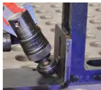
Clamping pad with spherical shape Clamping of corner profiles
