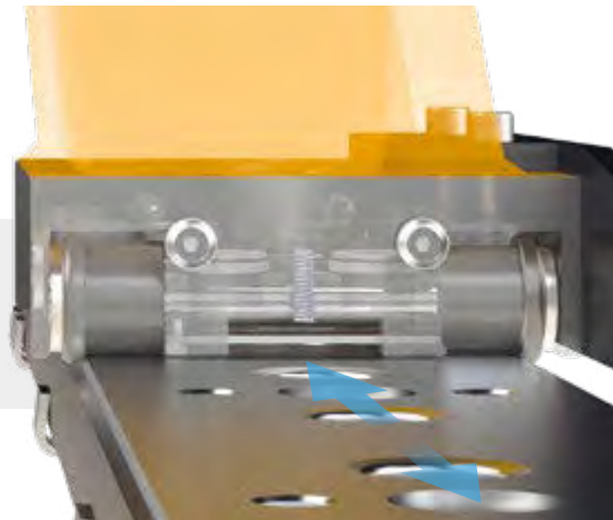
Spring-loaded lift = movement position (mounted on roller bearings so as to be movable)
