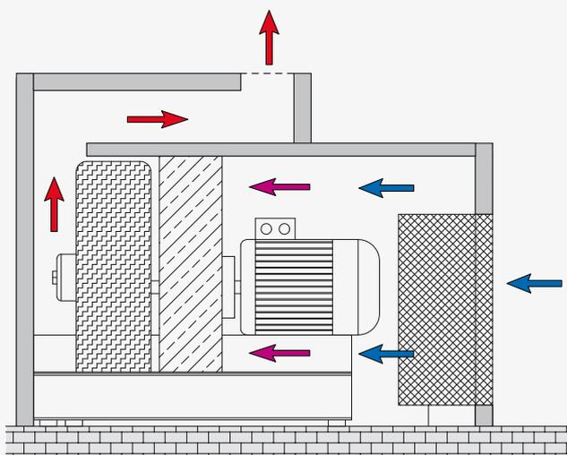
Sound insulation is also heat insulation, manufacturing quiet compressors **and** keeping them cool is the ultimate objective. With the ES concept, we have benchmark sound insulation **and** benchmark cooling. The cross sectional view of the ES housing illustrates the key features.
