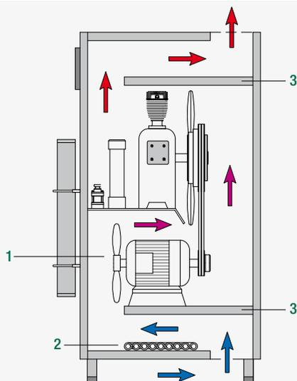
Sound insulation is also heat insulation, manufacturing quiet compressors **and** keeping them cool is the ultimate objective. With the ES concept, we have benchmark sound insulation **and** benchmark cooling. The cross sectional view of the ES housing illustrates the key features.
