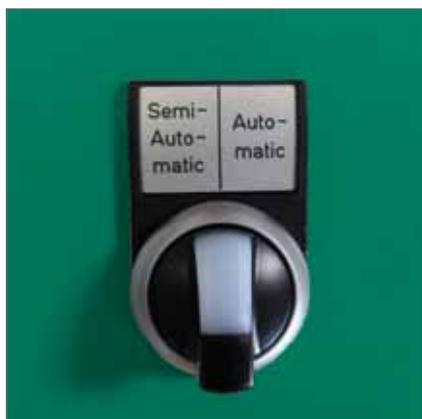
The auto start function allows operating the compressor optionally in automatic or semi-automatic mode by turning the selector switch.
