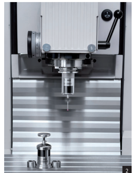
CNC dividing head (1), touch probe system and automatic tool measurement (2)
