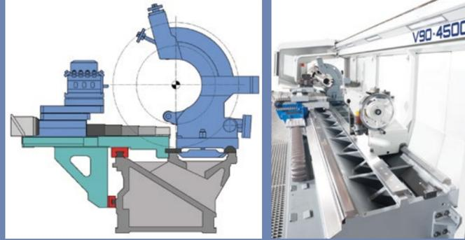
The machine takes its name from the four guideways along which the slides, tailstock and steady rest are moved. Precise, anti-friction bearings on a heavy-duty and torsion-resistant bed ensure the utmost positioning accuracy of the bed slides. The tailstocks and steady rest are precisely guided on hardened and finely-ground steel rails that are screwed on to the machine.
