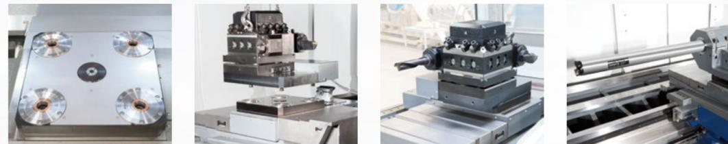
The design provides the straight-forward and precise change-over of the various tooling systems that range from tool turret, boring block and milling attachment through to a grinding unit on a quick-release plate.
