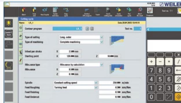
Cutting – extended parameters for machining
