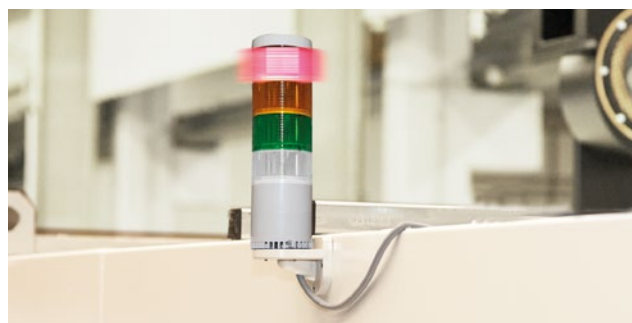
Signal lamp for visual indication of an alarm.
