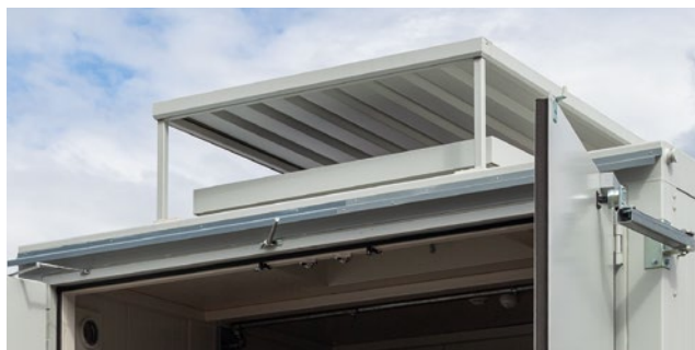
In the event of an explosion, the pressure is relieved via the roof panel. The weather protection prevents snow loads affecting operation
