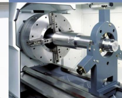
Pneumatically actuated front-end chuck with steady rest
