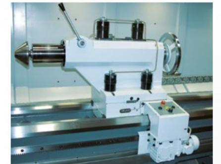
Tailstock with automated clamping and dedicated drive
