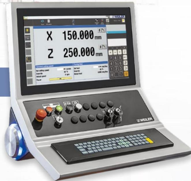
Even without prior programming knowledge, the smart WEILER software guides the operator through the programme. Using automated cycles, you can control the E-Series like a “manually operated” machine. Or you can completely program the workpiece contour with the assistance of the geometry processor that can even automatically calculate the points of intersection. For further information, please refer to the separate WEILER control brochure.
