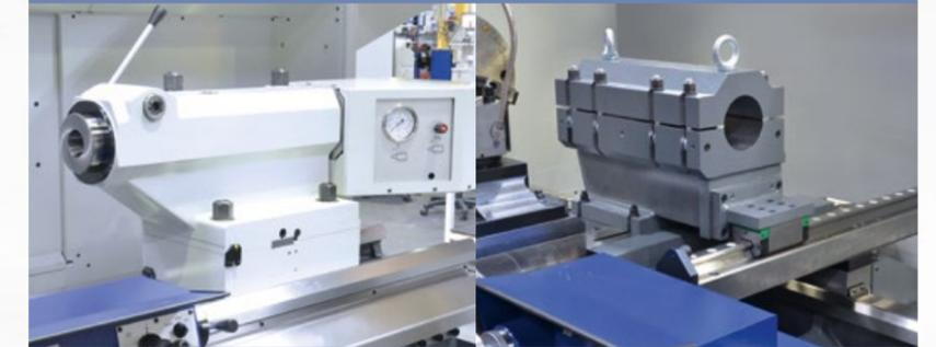
Tailstock with hydraulically actuated quill
