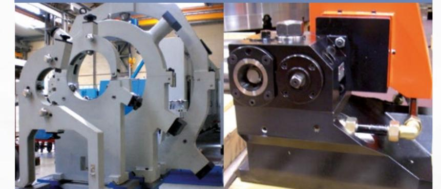
Steady rests for diameters up to 1,500 mm
