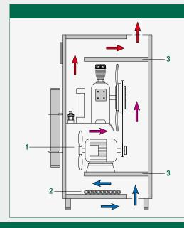
Sound insulation is also heat insulation, manufacturing quiet compressors **and** keeping them cool is the ultimate objective. With the ES concept, we have benchmark sound insulation **and** benchmark cooling. The cross sectional view of the ES housing illustrates the key features.
